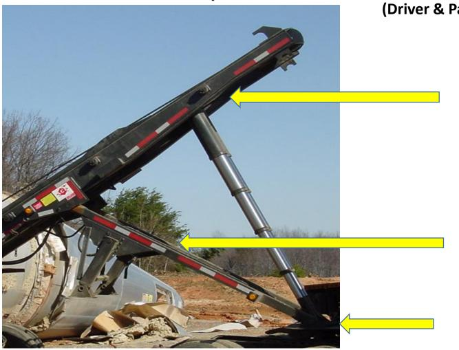
Ace uses TWO Tri-Angles working in tandem for unwavering stability (Driver & Passenger Side)
