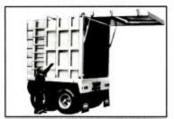
TOP-HINGED TAILGATE, hydraulically operated, assured fast, safe unloading. No "swinging door" problems when opening under load...or dumping on uneven terrain. Minimized stress on hinge areas reduces maintenance.
