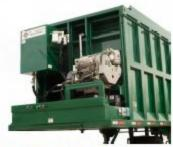
AUXILIARY ENGINE makes trailer a self-contained system...relieves tractor of being permanently "married" to the unit. Recommended for top-loading jobs...and for operations where the tractor is from a fleet not equipped with the PTO and hydraulic wet kit.
