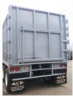
Standard rear tailgate of "doorin-adoor" design. Ejection door is side-hinged with heavy-duty locking mechanism on right or left as required. Lower door is designed to accommodate stationary packer... can be sized to handle a variety of makes.
